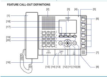
[1] Handset [2] Speaker [3] Color LCD Monitor [4] Status LED (orange / blue) [5] Directory cards and covers [6] Speed dial buttons (6) [7] Microphone [8] OFF button [9] ADJUST button [10] Menu navigation control button [11] Select button [12] Door release button [13] Transmit LED (blue) [14] TALK button [15] MONITOR button [16] Dial keys [17] PRIVACY button and LED (blue) [18] TRANSFER button and LED (orange) [19] LIST button and LED (blue) [20] SETTING button and LED (blue)
